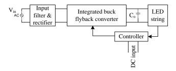
Fig. 4. Integrated single stage IBFC.
