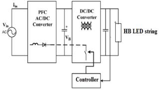
Fig. 3. Integrated single stage converter.
