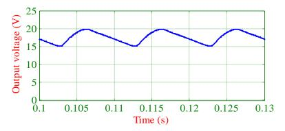
Fig. 15. Output voltage  $V_0$
