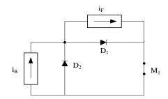
Fig. 8. Equivalent circuit during the conduction of  $M_1$
