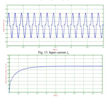
Fig. 14. Bulk capacitor voltage  $V_B$
