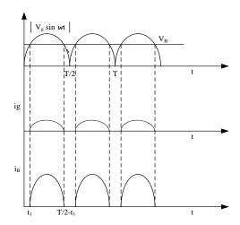
Fig. 10. Input voltage and current waveform of IBFC
