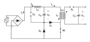
Fig. 7. Equivalent circuit of mode 2: v<sub>g</sub>>V<sub>B</sub> and M<sub>1</sub> is ON
