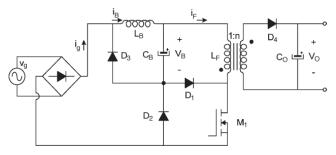
Fig. 5. Integrated buck flyback converter.
